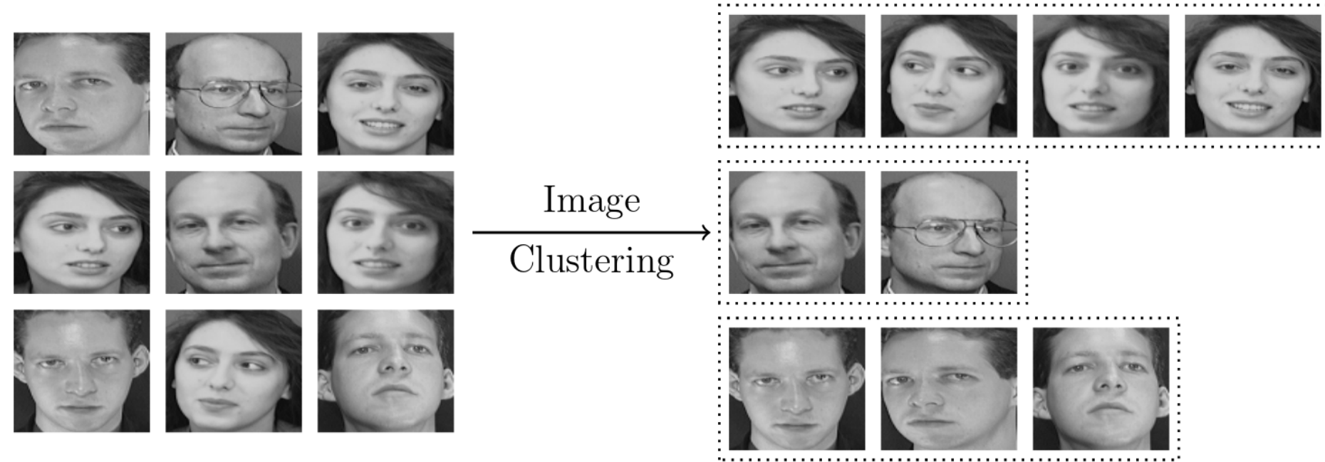
Fig. 1: Example of inputs/outputs of the image clustering problem
